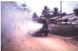
A Leco machine on a Landrover spraying with a pyrethroid insecticide to kill malaria vector mosquitoes resting inside or outside houses. (Malaria)
